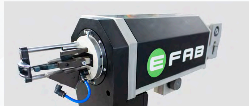
Mechanical tufting head with nonstop cut/loop changeover
